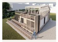
The HDU design consists of three major components: Living rooms, the Wintergarden and the Rooftop. It is built on a small plateau to represent the connection from the residential building to the vertical extension and includes the second story of the extension, including the Rooftop.
