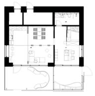
EFdeN VATRA prototype integrates into its plan the most important features from the Design Challenge, so in its composition, we find a one-level apartment module – adapted for people with disabilities, a greenhouse – with the possibility of extension into the outdoor terrace or into the apartment, the electrical and mechanical rooms, and the common room- which can be divided into four different spaces.
