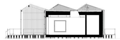
A vertical South-North section through the House Demonstration Unit. We can see the apartment module with the bathroom, and the attached greenhouse which can be opened into the interior of the house.
