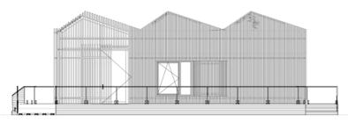
A vertical South-North facade of the House Demonstration Unit. We can see the eastern face of the prototype with the apartment's window and the secondary exit.
