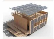
Like the Café Ada extension, the unit is divided into layers. The service layer includes the kitchen, the bathroom, the entrance area and the building utilities.
